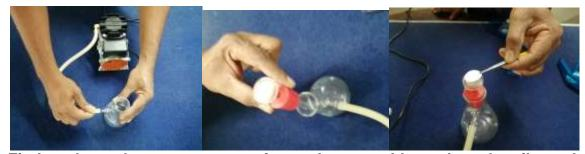
Fit the tube to the vacuum pump, insert the assembly to place the oil patch
